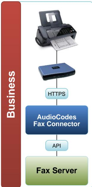
**1** Fax Connector is installed with the premise-based business fax server. Uses native API to connect to the fax server.
