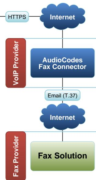
**3** Fax Connector is installed in the VoIP Provider's network. Connection to the 3<sup>rd</sup> party Fax Service provider is via email (T.37).
