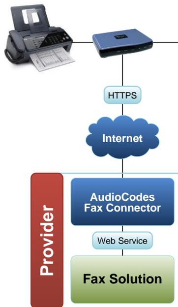
**2** Fax Connector is installed in the providers network. Uses Web Service API to connect to providers fax solution.
